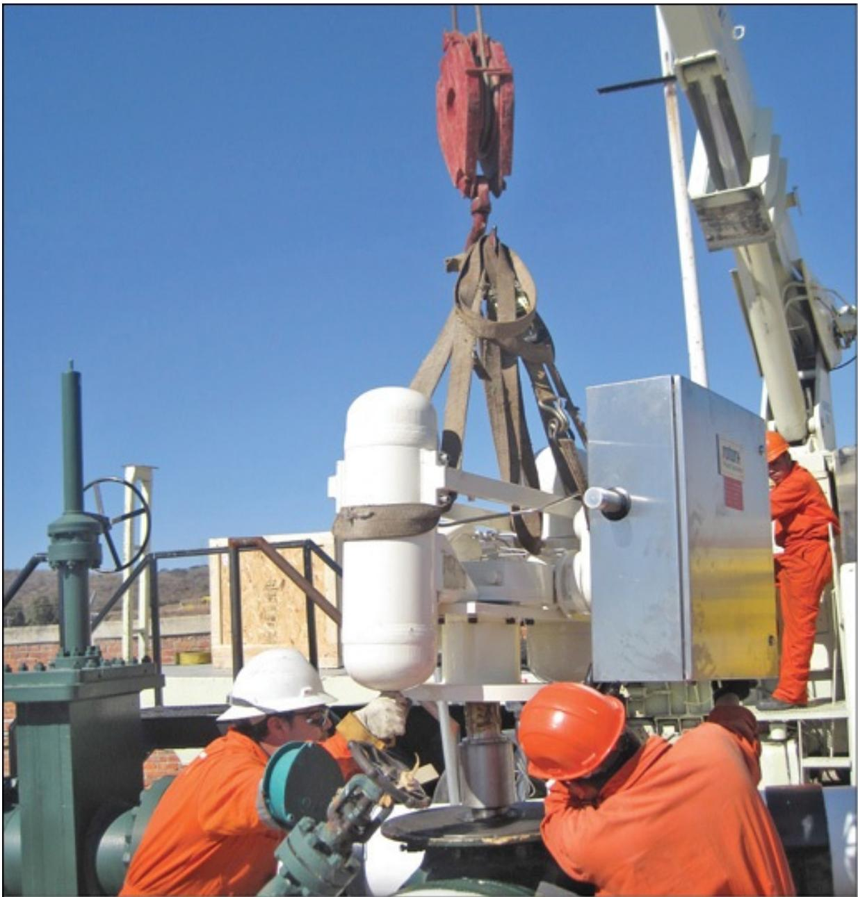
**Figure 11.1.a.** Mounting a fluid-powered actuator on a plug valve.
