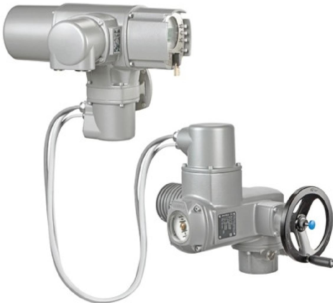
**Figure 5.4.1.b.** Motor starters and local push-button controls wall mounted for convenience and separate from the electric actuator. This configuration is also a method of isolating the actuator controls from vibration, temperature or other hostile elements at the valve. *Image courtesy of Auma.*
