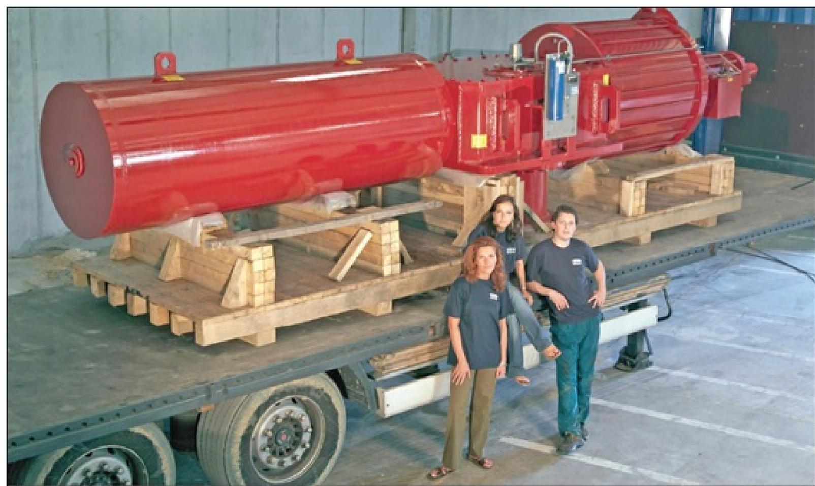
**Figure 6.2.1.2.f.** Large spring return scotch yoke pneumatic actuator.
