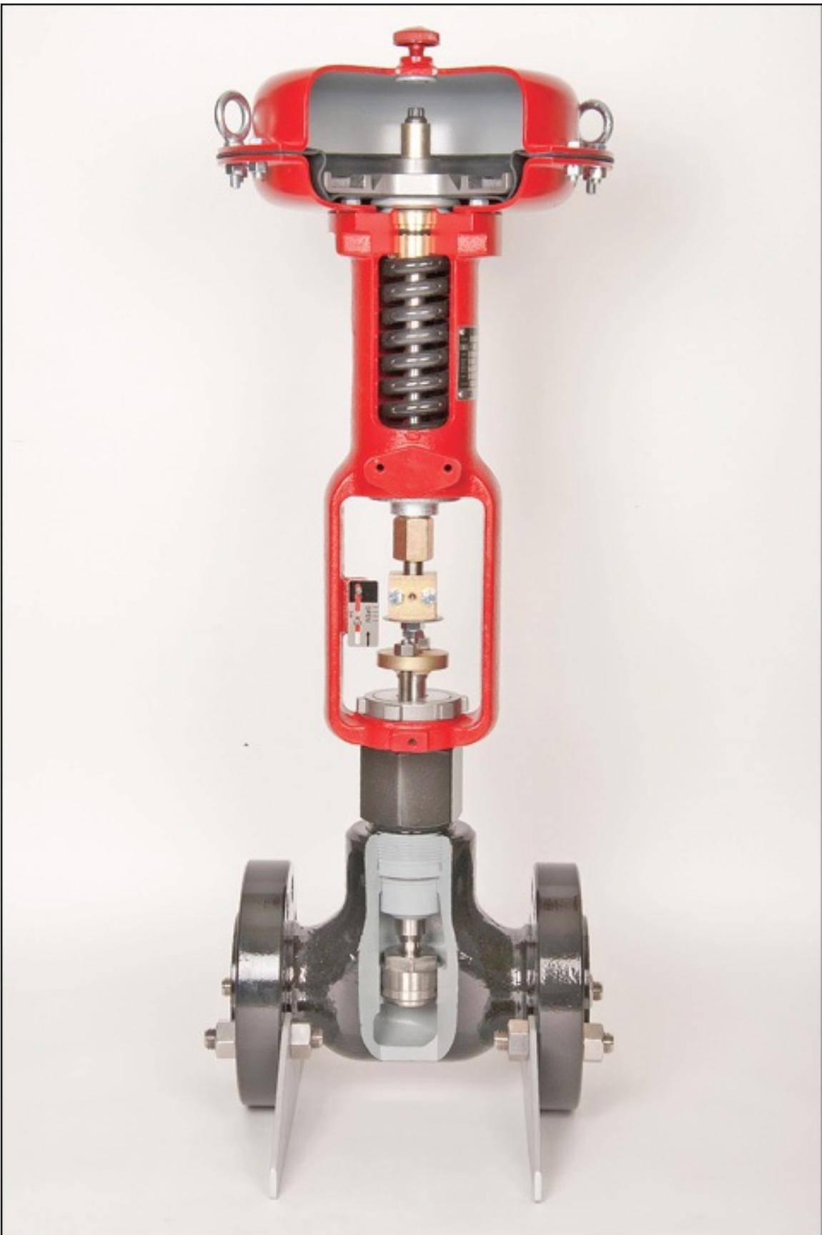
**Figure 6.2.3.1.a.** Linear pneumatic spring diaphragm actuator on a plug valve (air to open, spring close). *Image courtesy of Richards Industries.*
