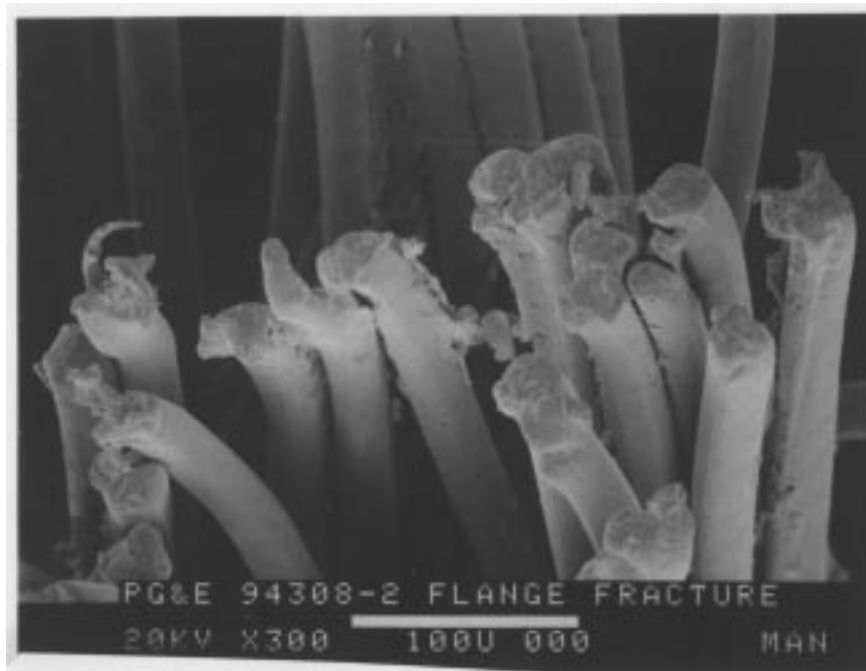
Figure 7-16 Nylon Fibers, Showing the Surface Details Resulting from Cutting Damage during Installation or Handling
