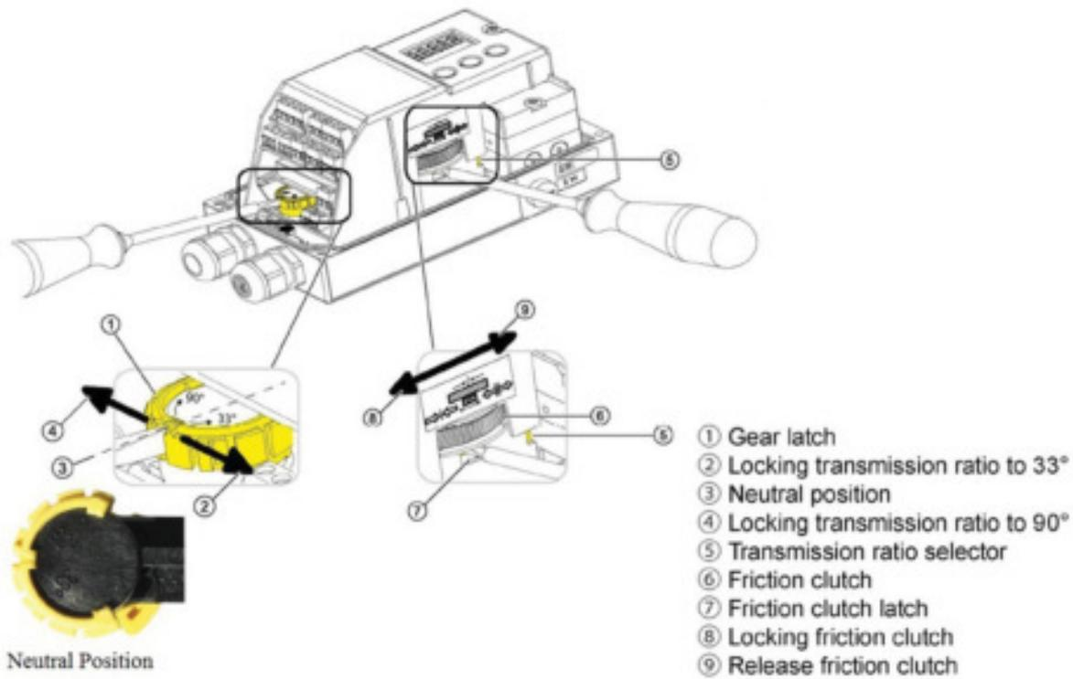
4. Set Transmission Ratio Selector (Slide Bar) according to the actuator's requirements:
