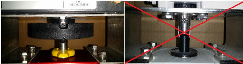
Figure 3-1 FlameProof coupler and SST coupler
