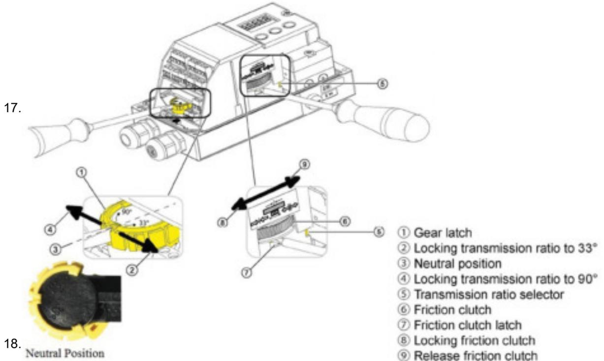
19. Lock the Friction Clutch; Move the slots left to lock (see ⑦ on image above)
