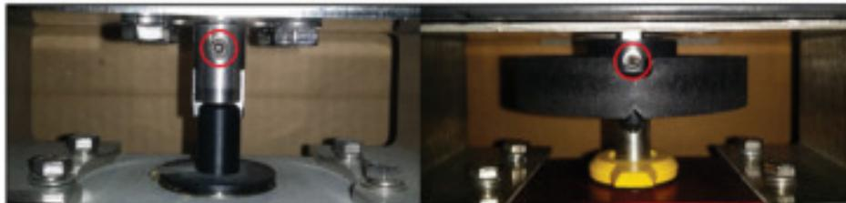
**Linear Applications – Verify all hardware is tight. If feedback solution has a *white cone style pin*, verify pin is compressed throughout all positions of the valve stroke.**
