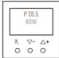
1. When the positioner is powered up for the first time, the display will flash **NOINI** (no initialization) on the bottom right of the screen.
