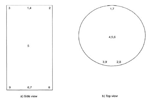
Figure H.2—Thermocouple locations—Cylindrical furnace (working zone)
