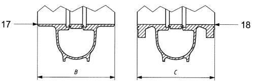
Figure 2 — Slab-gate/through-conduit rising-stem gate valve
