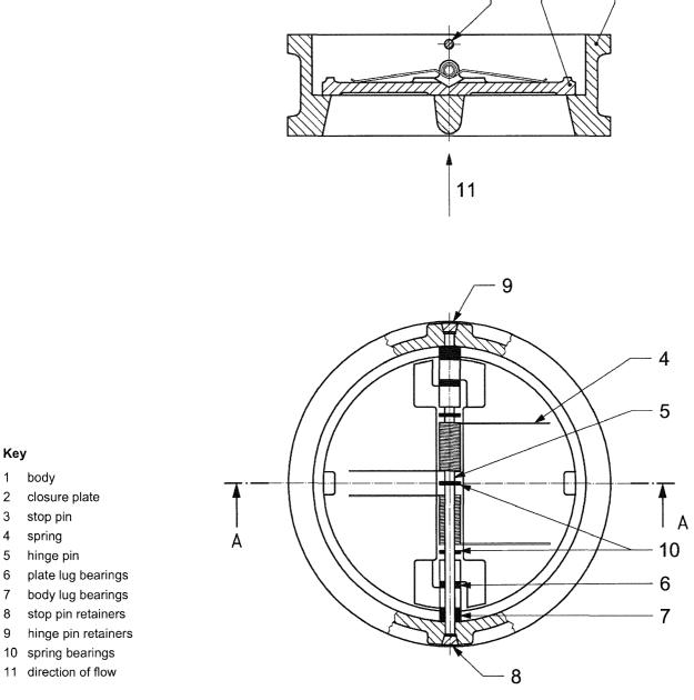
Figure 10 — Typical dual-plate wafer-type check valve, long pattern
