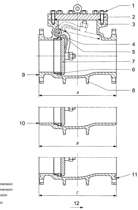
Figure 8 — Full-opening swing check valve
