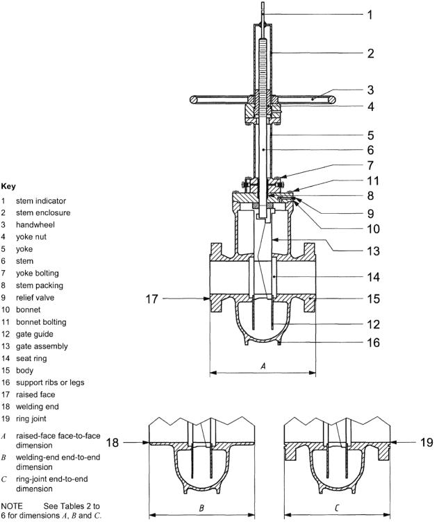
Figure 1 — Expanding-gate/rising-stem gate valve
