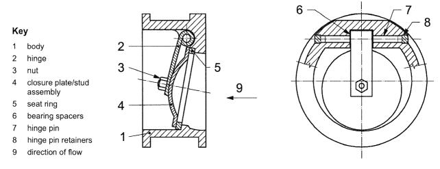
Figure 9 — Single-plate wafer-type check valve, long pattern
