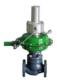
**ZZVMP** self-regulating type nitrogen seal valve is composed of control valves, actuators and pilot, is a kind of no extra energy, using the pressure as power source, modulated medium itself to automatically adjust the pressure constant of energy-saving products, the valve control is twice precise as general self-reliance type pressure regulating valve, suitable for requiring higher control precision
